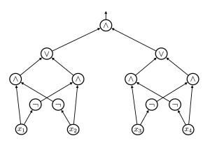
The output gate is the gate at the very top with an arrow that links to nothing. The circuit outputs 1 if and only if  $x_1 \neq x_2$  and  $x_3 \neq x_4$ .
